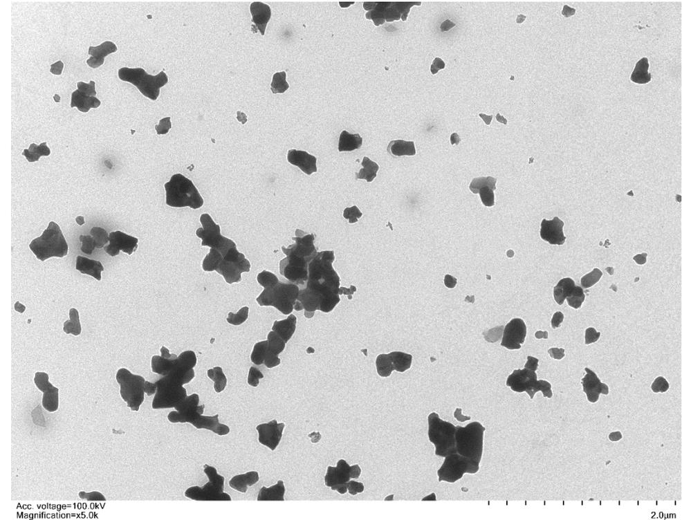
In this hydrophilic solution (NMP), there're some secondary particles to be observed with the aggregated granule sizes larger than 1,000nm.
