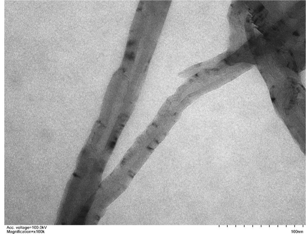
Each of MWCNTs could be observed with a few node-like structures along the nanotube.
