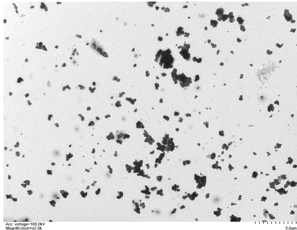
The nanoparticles in NMP were likely comprised of two groups, primary (Individual) and secondary (Originally aggregated) particles.
