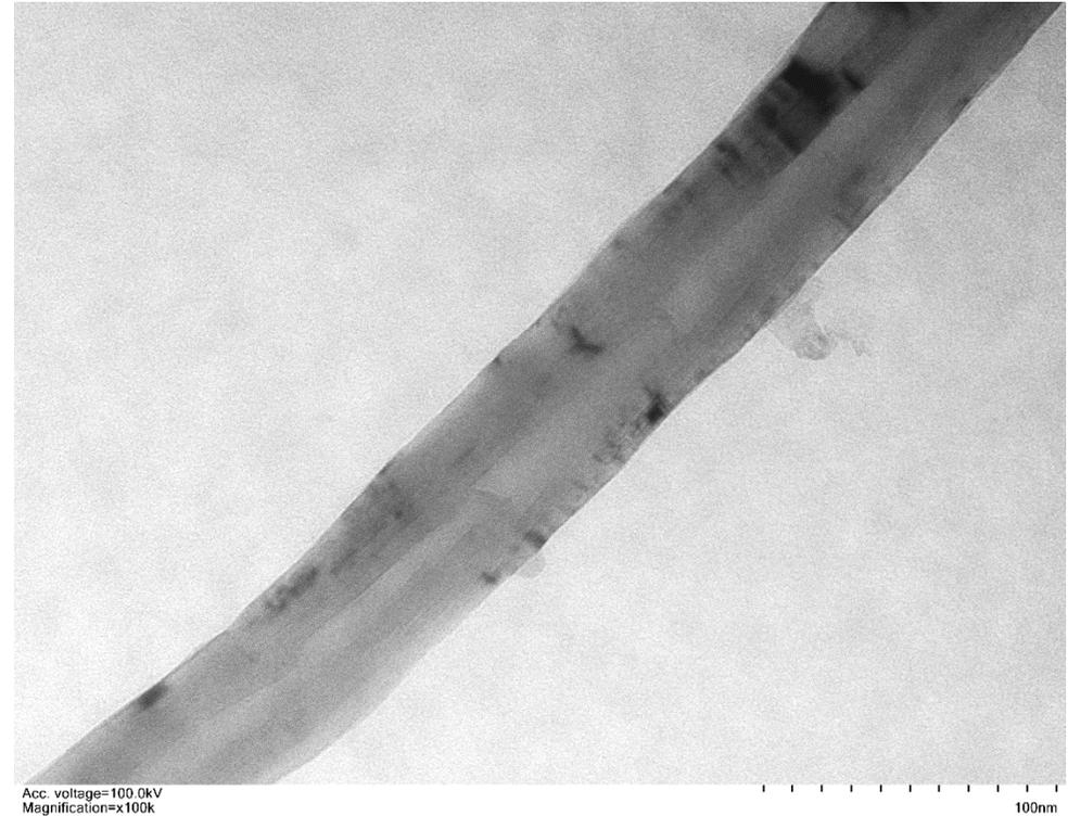
By the imaging results under a larger magnification, the tubular microstructures of MWCNTs were all with multiple walls to form their outer shells.
