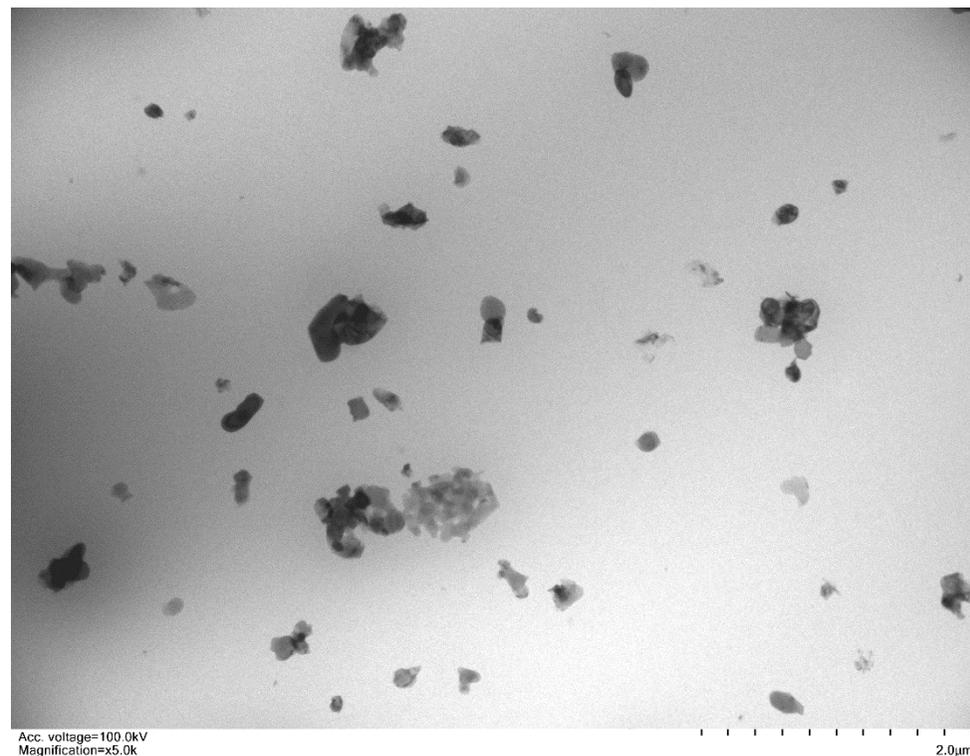
As shown the TEM imaging results, Al<sub>2</sub>O<sub>3</sub> nanoparticles were evenly distributed in NMP solution basically.
